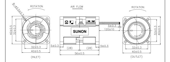
NOTE: 1. LEAD WIRE: UL1571 #28AWG INLET
