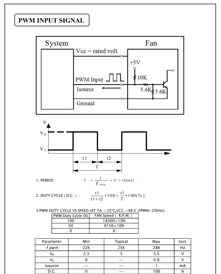
\* The speed is default to be maximum if PWM input pin is unconnected. \* Min. start up duty cycle is 20%.
