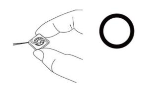
Don't pull fan with lead wires.
