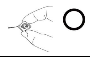
Don't pull fan with lead wires.
