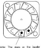
Note: The glues on the impeller is for impeller balance.
