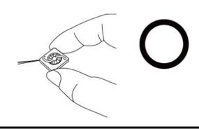
Don't pull fan with lead wires.
