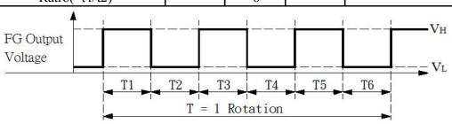
T= T1+T2+T3+T4+T5+T6=1 Rotation  $T=\frac{60}{rpm}$
