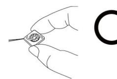
Don't pull fan with lead wires.
