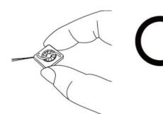
Don't pull fan with lead wires.
