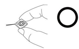
Don't pull fan with lead wires.
