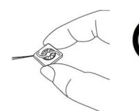
Don't pull fan with lead wires.
