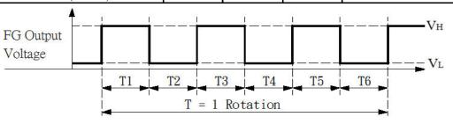
T= T1+T2+T3+T4+T5+T6=1 Rotation  $T=\frac{60}{rpm}$
