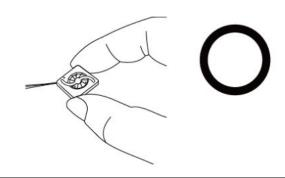
Don't pull fan with lead wires.
