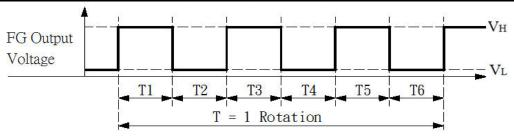
T= T1+T2+T3+T4+T5+T6=1 Rotation  $T=\frac{60}{rpm}$
