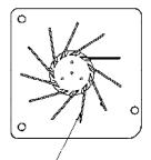
Note: The glues on the impeller is for impeller balance, Please don't remove it.
