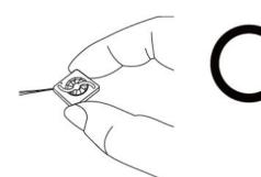
Don't pull fan with lead wires.
