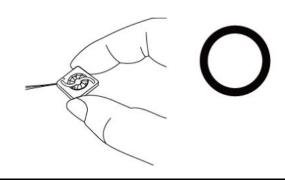
Don't pull fan with lead wires.
