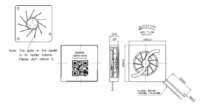
Marking (By laser): SUNON UB3F3-XXXX:Model name Production serial number:0Y17xxxxxx 0:Printing Plant Code Y:Manufacture Plant 17:Year.2017=17 xxxxxx: Producing Lot No. QR code :Content according to SUNON QR code specification
