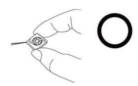
Don't pull fan with lead wires.
