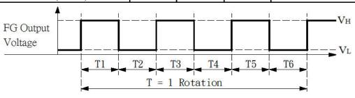
T= T1+T2+T3+T4+T5+T6=1 Rotation  $T=\frac{60}{rpm}$
