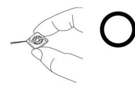
Don't pull fan with lead wires.
