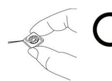
Don't pull fan with lead wires.
