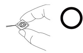
Don't pull fan with lead wires.
