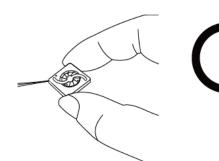
Don't pull fan with lead wires.
