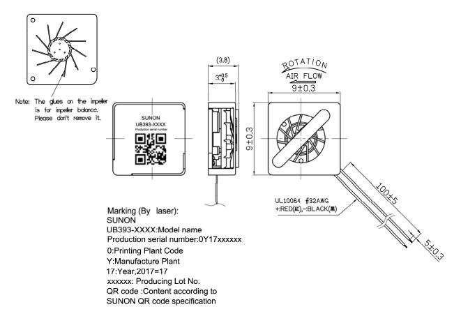
Sunon standard sample exclude the connector. If there is any request for connector, please advise in advance. About recommend connector, SUNON recommend the following models for SUNON Mighty Mini Fan/Blower: 1.(JST) SUR series connector: 02SUR-32S / 03SUR-32S / 04SUR-32S.
