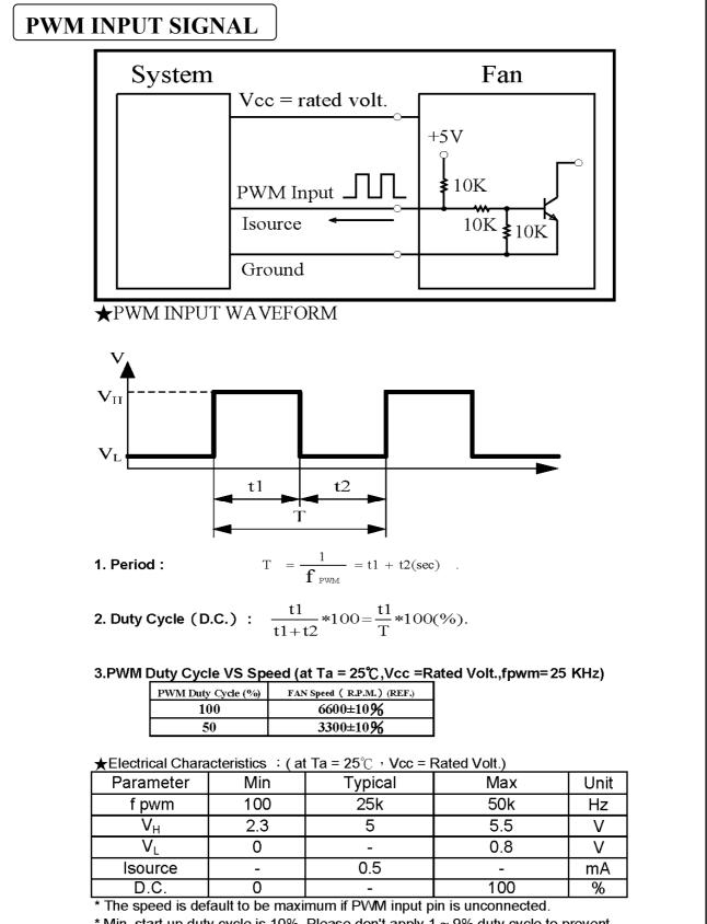
\* Min. start up duty cycle is 10%. Please don't apply 1 ~ 9% duty cycle to prevent unstable fan speed.
