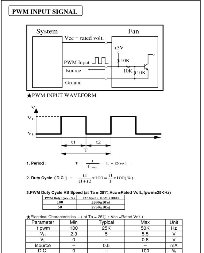
\* The speed is default to be maximum if PWM input pin is unconnected.
