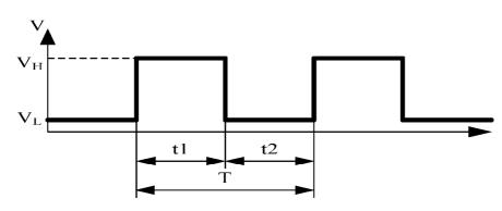
$$T = \frac{1}{f_{\text{PWM}}} = t1 + t2(\text{sec}) \quad .$$
