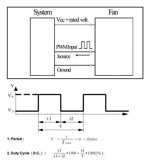
3.PWM Duty Cycle VS Speed (at Ta = 25°C, Vcc =Rated Volt., fpwm= 25 KHz)
