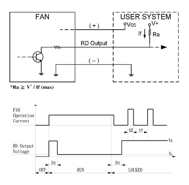
★Electrical Characteristics  $\therefore$  Vcc =12V , (at Ta = 25°C)
