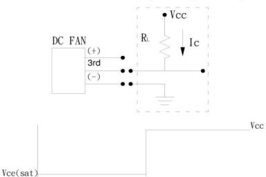
$\begin{tabular}{l} Vcc=13.8V(Max) \\ Ic=5mA(Max) \\ RL \geqq Vcc/Ic \\ \end{tabular}$  Locked
