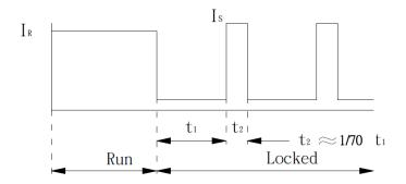
3rd wire signal Run : Square Wave Locked : V<sub>H</sub> or V<sub>L</sub>
