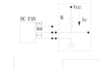
$Vcc = 13.8V(Max) \\ Ic = 5mA(Max) \\ RL \ge Vcc/Ic \\ Run \qquad Locked$
