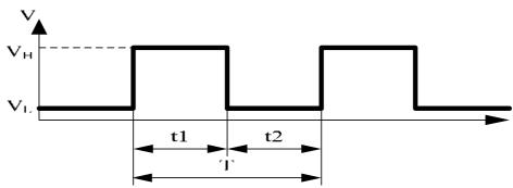
$$T = \frac{1}{f_{\text{PWM}}} = t1 + t2(\text{sec}) \quad . \label{eq:T_pwm}$$
