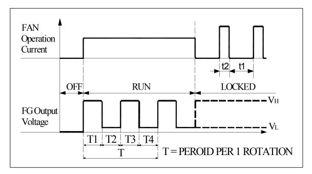
★Electrical Characteristics : (  $Ta = 25^{\circ}$ C , Vcc = Rated Volt.)
