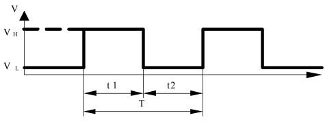
$$T = \frac{1}{f_{\text{PWM}}} = t1 + t2 (sec) \quad . \label{eq:T_PWM}$$
