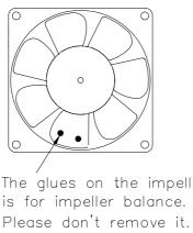
Note: The glues on the impeller is for impeller balance.
