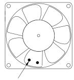
Note: The glues on the impeller is for impeller balance.
