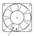
Note: The glues on the impeller is for impeller balance. Please don't remove it.
