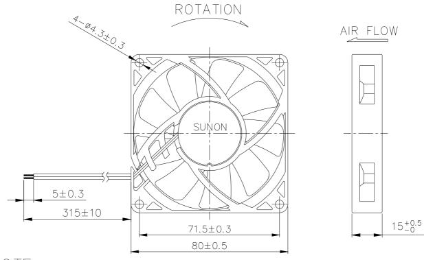
NOTE: 1.LEAD WIRE:UL1007 #24AWG RED WIRE----(+) BLACK WIRE----(-) 2.FRAME TYPE:RIB
