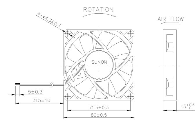
NOTE: 1.LEAD WIRE:UL1007 #24AWG RED WIRE----(+) BLACK WIRE----(-) 2.FRAME TYPE:RIB
