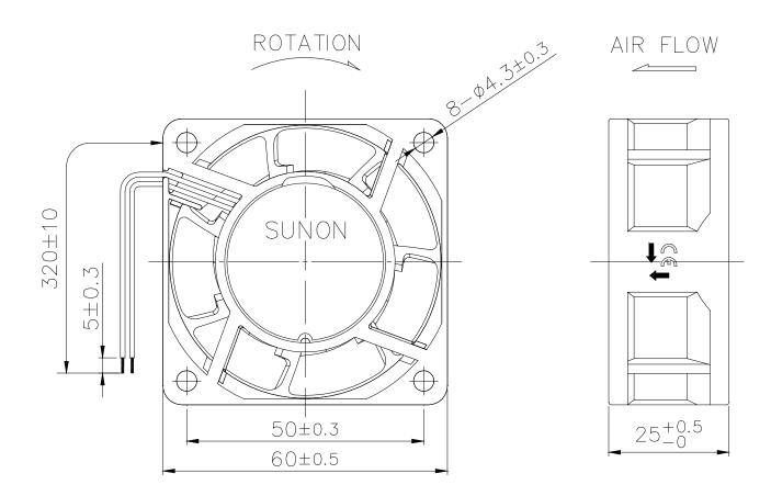
NOTE: 1.LEAD WIRE: UL3266 #24AWG GRAY 2.FRAME TYPE: FLANGE
