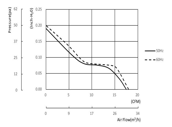
NOTE: The airflow and static pressure are measured with SUNON's specific fixture.
