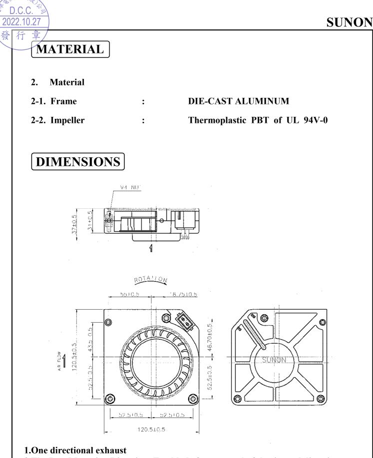
2. The Best Mounting Direction: Fan blade face up or shaft horizontal direction.
