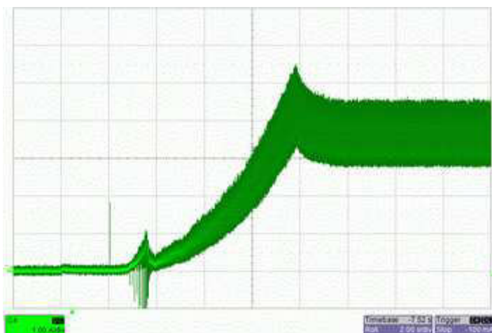
Start-up current @ 48 V ( I = 1\text{A/div} ; t = 2\text{s/div} )
