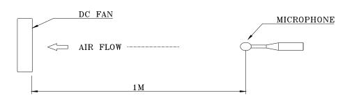
NOISE IS MEASURED AT RATED VOLTAGE IN FREE AIR IN ANECHOIC CHAMBER WITH MICROPHONE AT A DISTANCE OF ONE METER FROM THE FAN INTAKE.
