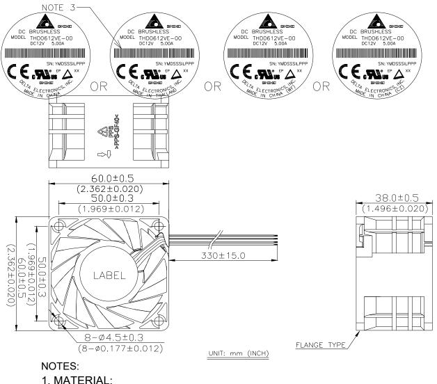
LEAD WIRE : UL1007 AWG#26 BLACK WIRE (GND)-----(AWG#26) RED WIRE (+12V))-----(AWG#26) YELLOW WIRE (TACH RPM))------(AWG#26) BLUE WIRE (PWM))------(AWG#26)
