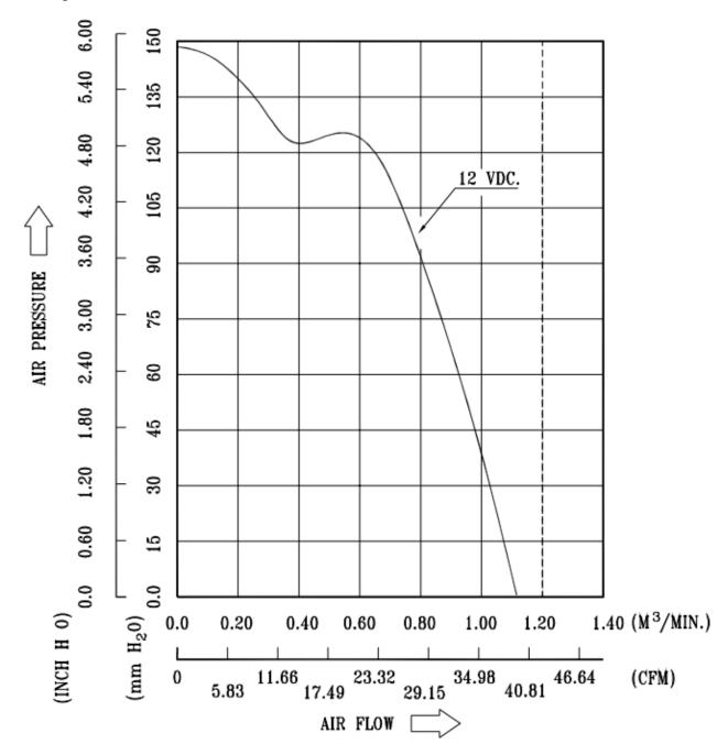
\*TEST CONDITION: INPUT VOLTAGE-----OPERATION VOLTAGE
