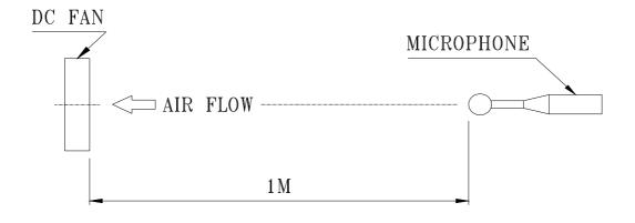
NOISE IS MEASURED AT RATED VOLTAGE IN FREE AIR IN ANECHOIC CHAMBER WITH MICROPHONE AT A DISTANCE OF ONE METER FROM THE FAN INTAKE.
