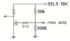
13-1. THE FAN SPEED WILL DEFAULT TO MAXIMUM WHEN THE SPEED CONTROL INPUT IS LEFT UNCONNECTED.
