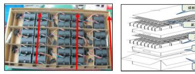
12-3-2. MAKE SURE DESICCANT, QUANTITY AND P/N IS CORRECT BEFORE PACKING.
