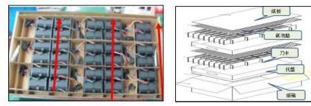
12-3-2. MAKE SURE DESICCANT, QUANTITY AND P/N IS CORRECT BEFORE PACKING.
