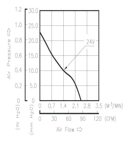
\*TEST CONDITION: INPUT VOLTAGE-----OPERATION VOLTAGE
