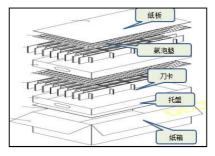
14-3-2. MAKE SURE DESICCANT, QUANTITY AND P/N IS CORRECT BEFORE PACKING.
