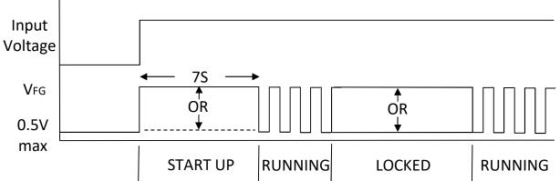
SINCE THIS FAN HAS 4.0 SEC BRAKE FUNCTION AND 3-PHASE SENSORLESS TECHNOLOGY, THE FG SIGNAL WILL APPEAR AFTER POWER ON 7.0 SEC
