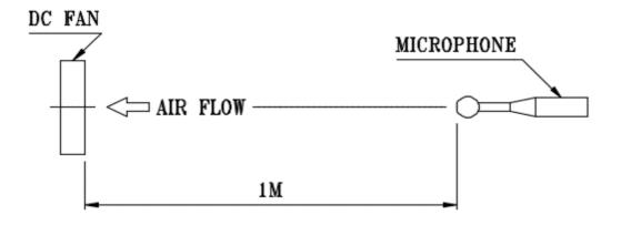
NOISE IS MEASURED AT RATED VOLTAGE IN FREE AIR IN SEMI-ANECHOIC CHAMBER WITH MICROPHONE AT A DISTANCE OF ONE METER FROM THE FAN INTAKE.
