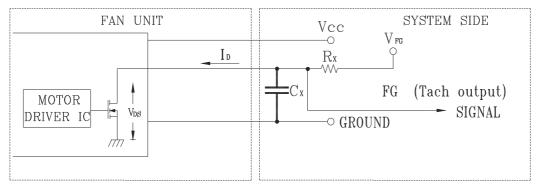
GENERAL CONDITION: VFG is 3.3V, Rx is 8.2Kohm, and Cx is 4nF. CAUTION: THE FG SIGNAL LEAD WIRE MUST BE KEPT AWAY FROM "+" LEAD WIRE & "-" LEAD WIRE.
