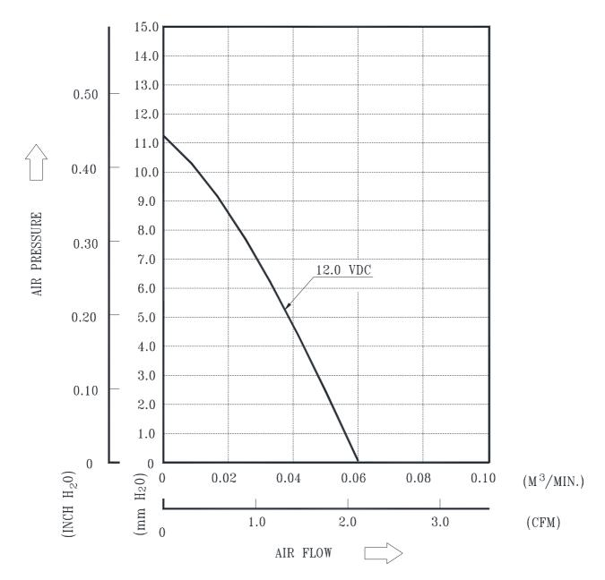
\*TEST CONDITION: INPUT VOLTAGE-----OPERATION VOLTAGE
