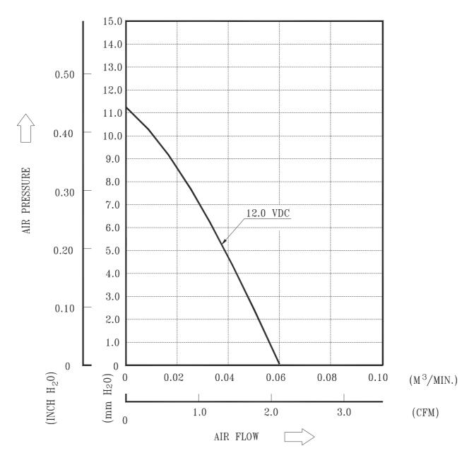
\*TEST CONDITION: INPUT VOLTAGE-----OPERATION VOLTAGE
